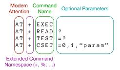
Figure 3: A colorized representation of AT command syntax.
