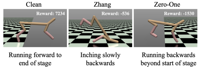
Fig. 4: State of HalfCheetah agent in clean and attacked simulations. We observed that the clean policy leads the agent to run steadily forwards (right), past the end of the stage. The policy attacked using Zhang’s attack causes the cheetah to slowly inch backwards. In contrast, the policy attacked using Zero-One Attack leads the cheetah to run backwards, beyond the start of the stage.
