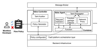
Figure 2: A reference architecture of VALVE.
