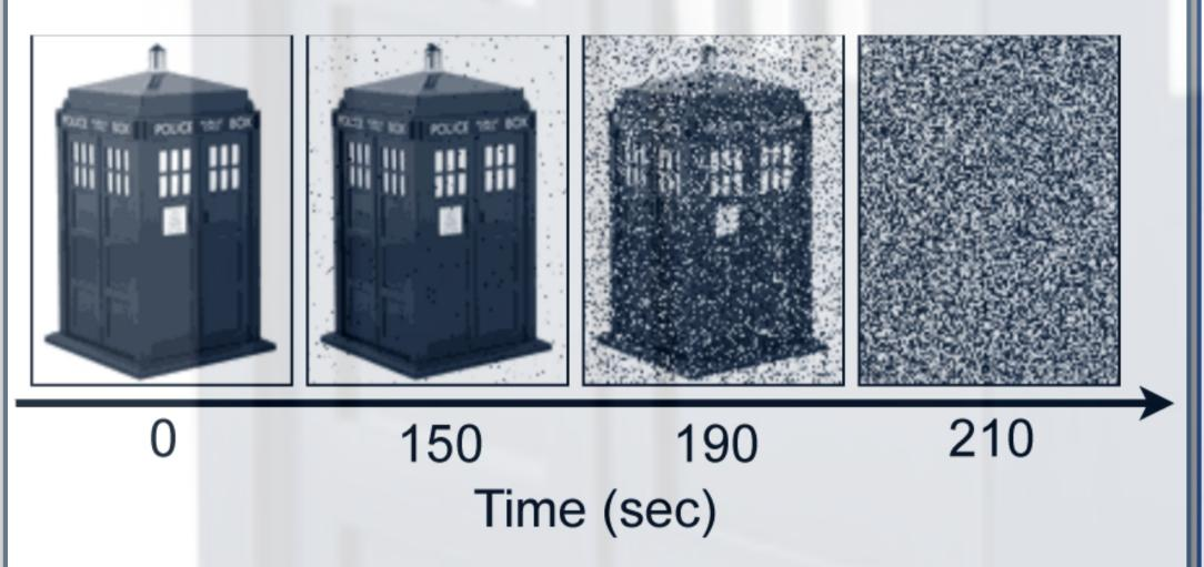
SRAM is a **volatile memory** that loses data in the absence of power. This loss of data is gradual and depends on the circuit's specifications, capacitance, and temperature. TARDIS derives a notion of time from the gradual data loss.
